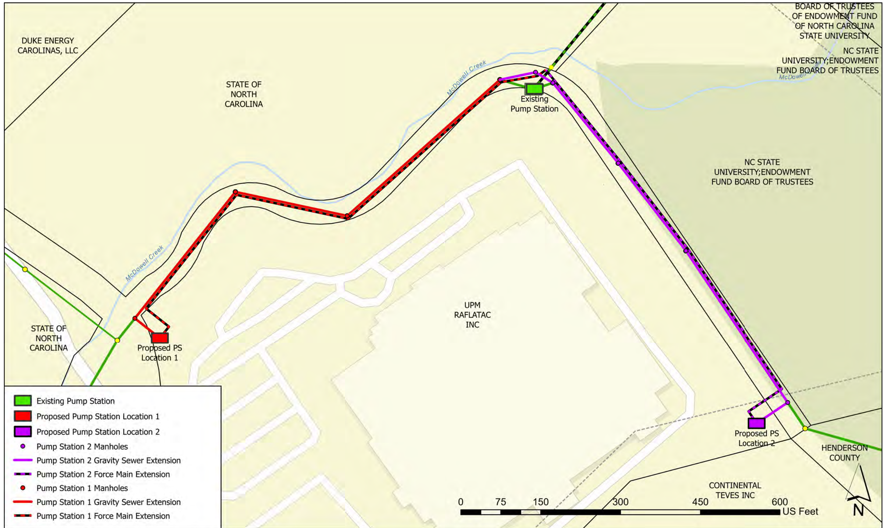
Attachment B. Proposed Pump Station Locations
