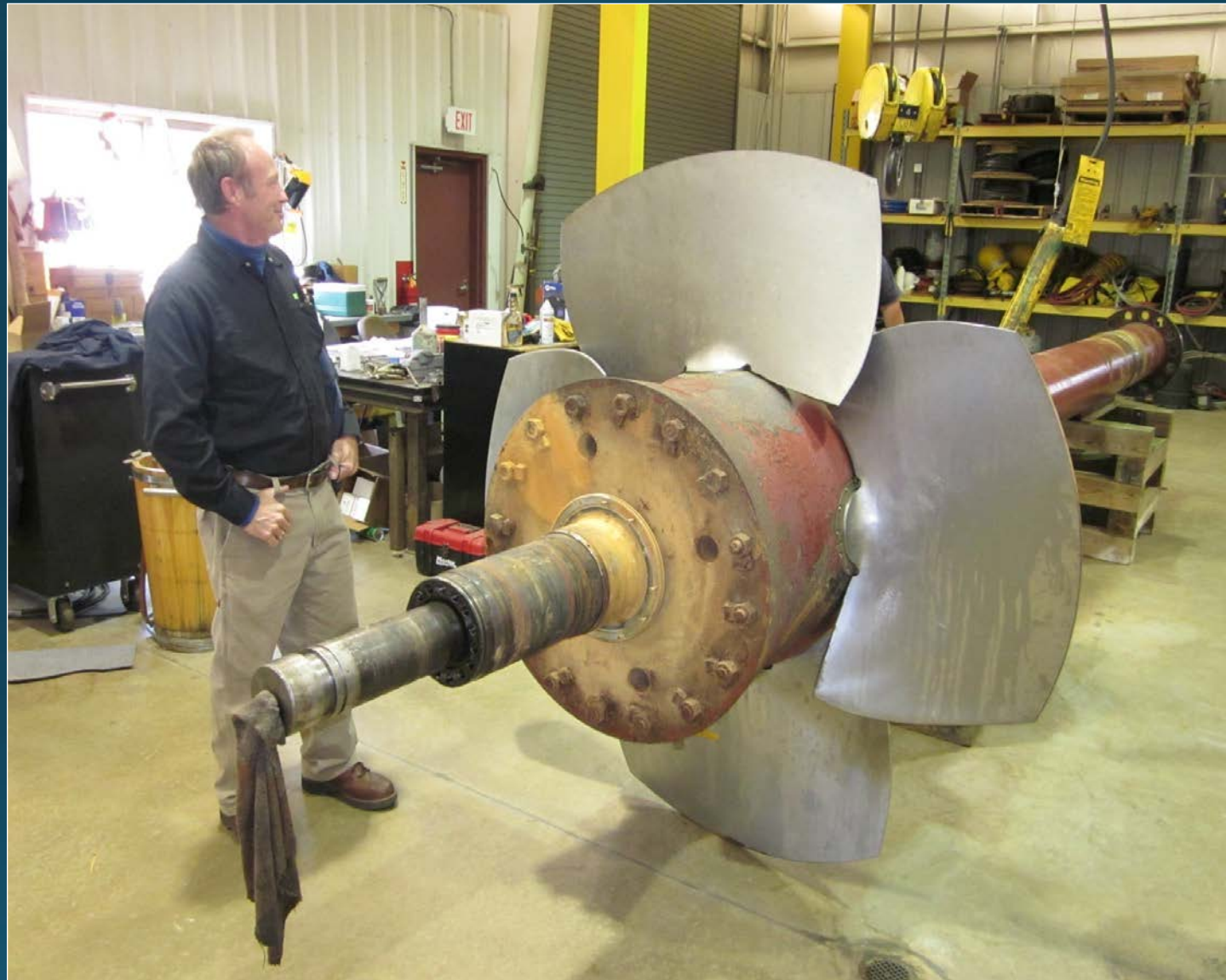
One of three turbine blades - variable pitch.
