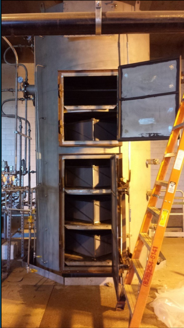
Three stories up - sorbent panel layers.
