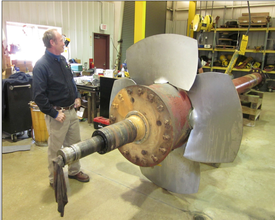
One of three turbine blades - variable pitch.
