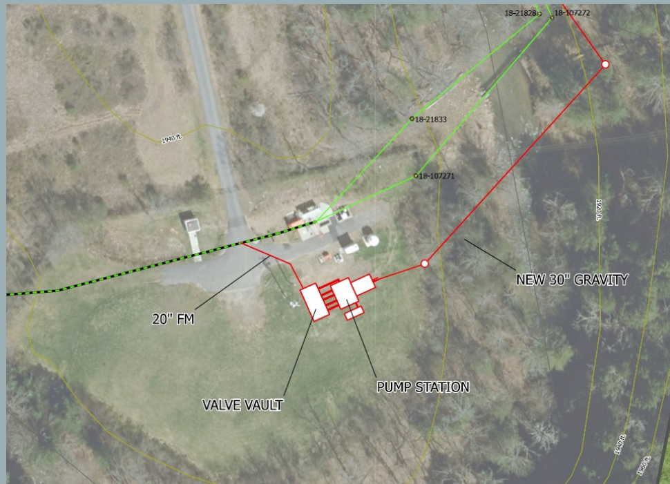
Conceptual design schematic at W'ville PS No. 1
