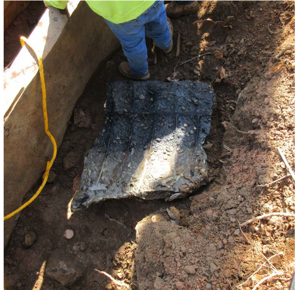
Section of pipe "crown" with reinforcing bars exposed
