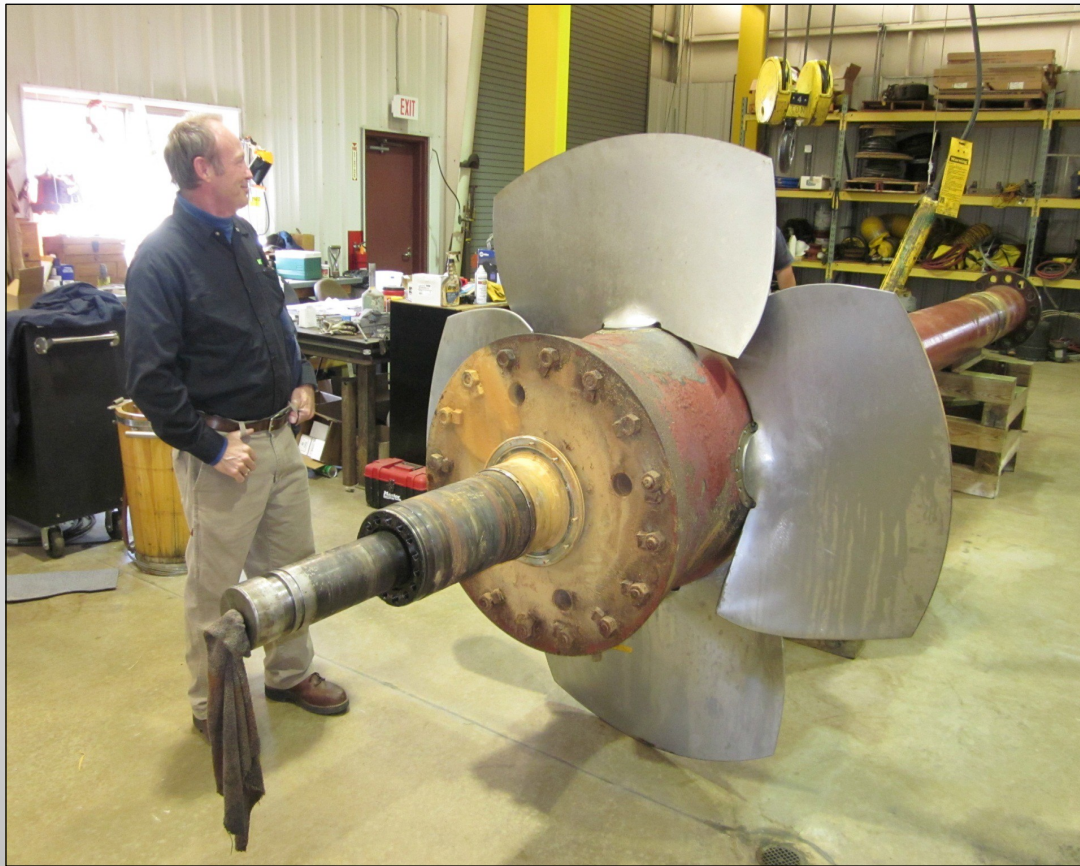
One of three turbine blades - variable pitch.
